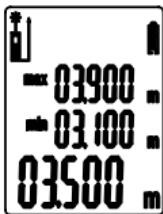
Continuous measurement automatically switch off after 100 times measurements (about 30 seconds).
