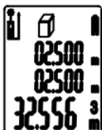
After taking the third measurement, the volume is automatically calculated and displayed. The last individual measured value is indicated at the middle line in the display, while the final result is shown at the bottom.
