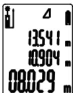
After completing the second measurement, the height of the building is calculated automatically. The last individual measured value is indicated at the middle line in the display, while the final result is indicated at the top.
