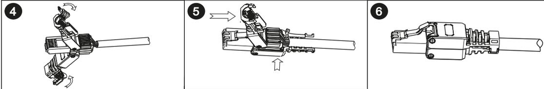
**4** ACCORDING CABLE EXTERNAL DIAMETER PUT PLASTIC WIRE GUARD INTO HOLDER HOLE LIKE THE ARROWHEAD
